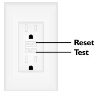
detects any disruption it will trip and shut the power off, which can only be regained by pressing the reset button. It is good to periodically check these plugs by pressing the test
